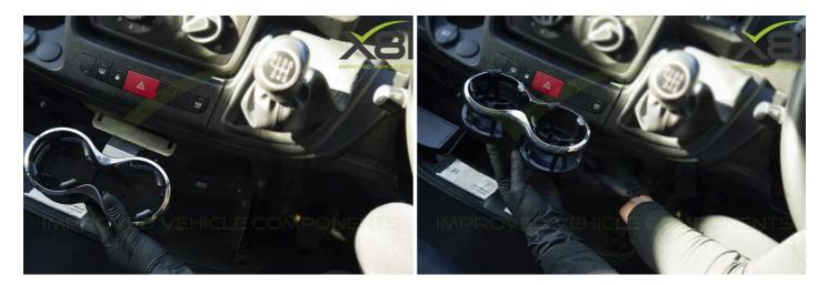
Slide the cup holder bracket to sit on the loosened threads of the screws.
