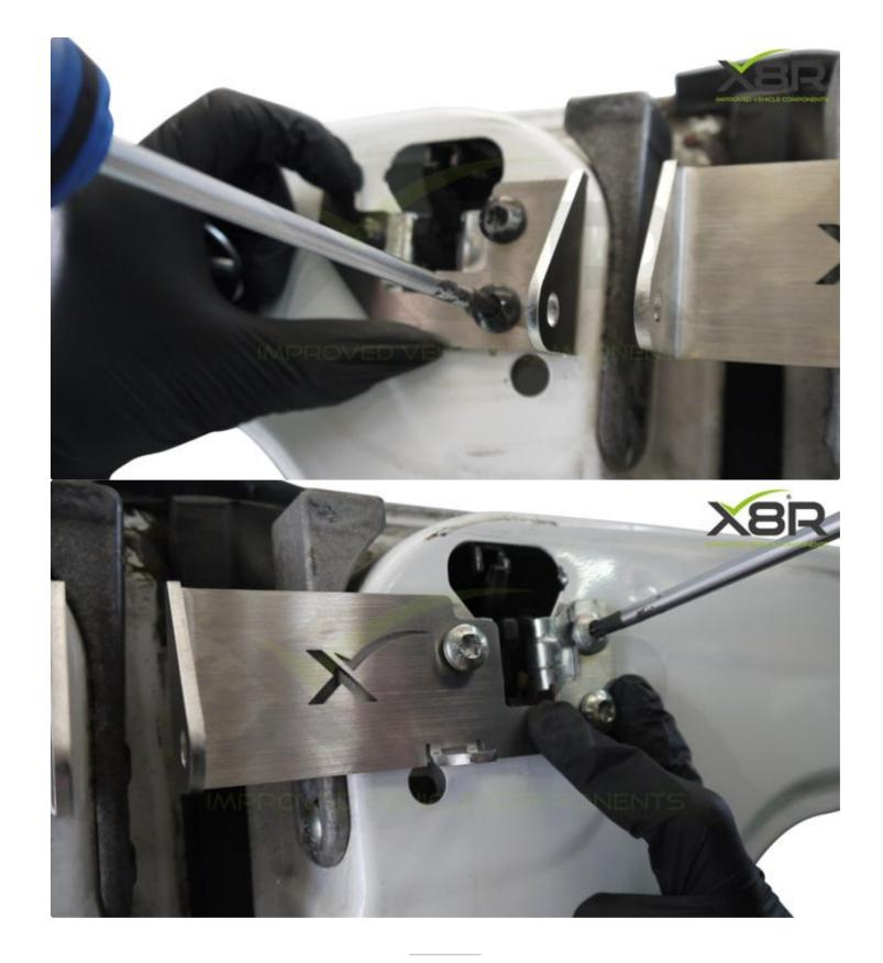
**Step 5: Line Up and Tighten the Brackets**
