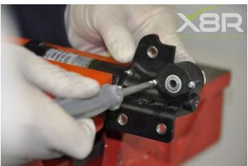
Step 3: Remove the motor cover and the old gear Remove the 2x Philips screws from the cover.
