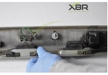
ssan Qashqai Tailgate Boot Handle Repair Clip Kit Clips 2006 -2013 for Snapped Handle Clips Install Instruction Guide: Page
