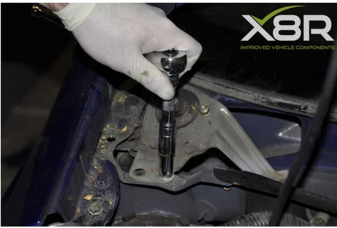
**Step 6: Remove the old wiper linkage push rods**
