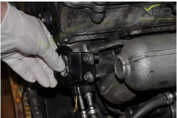
**Step 4: Remove Fuel Temperature Sensor**
