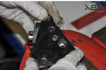
Step 13: Refit Fuel Strainer And O-ring
