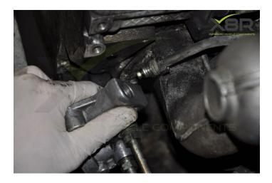
Step 9: Remove Fuel Line Studs And Replace O-rings
