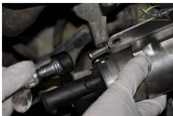
Step 7: Remove Fuel Pressure Regulator Block
