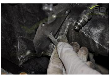
Step 14: Refit Fuel Pressure Regulator Block
