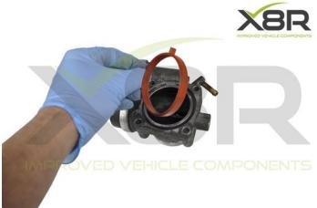
**Step 16: Remove Supercharger Air Supply Tube**
